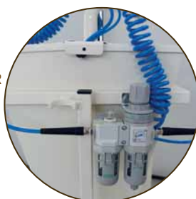
AIR REGULATOR FOR THE VIBRATING SYSTEM
