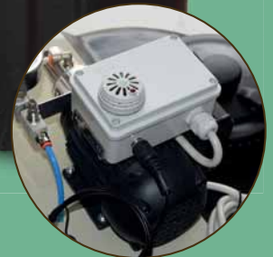
LIQUID LEVEL CONTROL SYSTEM
