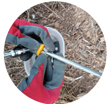
6. PLACEMENT OF THE LINSEED OIL GLAZING PUTTY AT THE BASE OF THE NEEDLE
